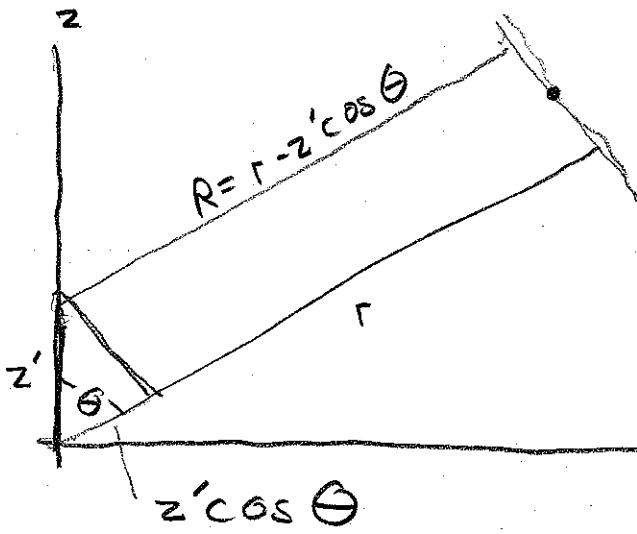
$kz' \cos \theta$  is just the phase difference of a small current element located at  $z'$  w.r.t. the origin
