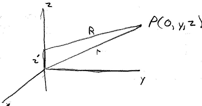
By symmetry, there should be no  $\phi$  dependence so we can look at any  $\phi$  angle
